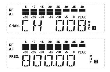
With the "▲" or "▼" buttons you can directly switch between the factory-preset frequencies (Channels presets). The display starts flashing by indicating that your selection is active. Press SET button to record your setting.
