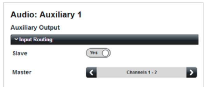
Auxiliary Outputs are by default mono. When one is slaved to a stereo pair of channels, its source becomes a mono sum of the signals in the two channels. Alternative, mono amplifier channels will be available as sources via the **Master** selector for Auxiliary Outputs when they are not in Slave mode is unchanged: any Line Input (or **off**) may be selected.
