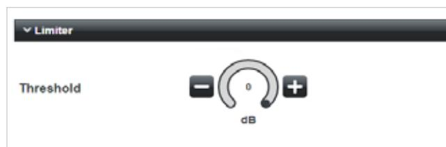
The limiter is a simple peak-detecting type. Limiting action commences when the signal level exceeds the setting of the **Threshold** control; click the + and – buttons to adjust. This has a range of 24 dB in 1 dB increments. Limiting action triggered by the signal level exceeding the threshold has finite attack and release times, which have been optimised for most normal types of programme material.
