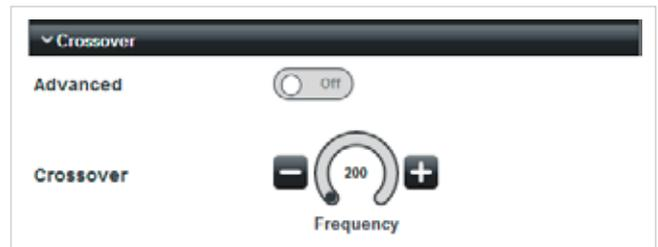
With **Advanced** set to **Off**, a default crossover is implemented, adjusted by the Frequency control: the crossover type is a Linkwitz-Riley filter with a slope of 24 dB/octave. The range of adjustment is the full audio range of 20 Hz to 20 kHz. Signal content above the crossover frequency will be routed to the **HF Speaker** channel (in this example, Channel 3) and content below the crossover frequency to the **LF Speaker** channel (in this example, Channel 4).
