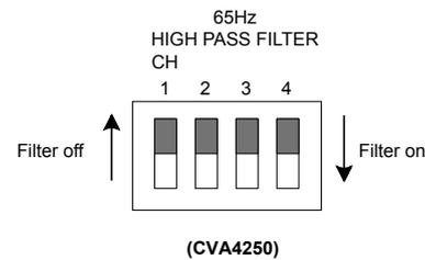
The factory default filter frequency is 65 Hz, which should be satisfactory for many installations; however the frequency can be adjusted over the full audio bandwidth from the web browser pages. Note also that the DIP switch may be disabled, on a per-channel basis, from the web browser pages.
