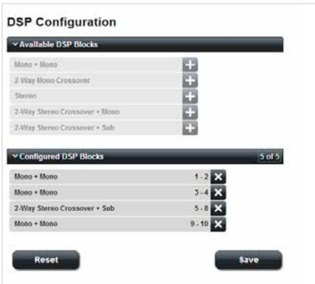
This configuration uses four amplifier channels for the crossover: like the 2-Way Stereo Crossover + Mono DSP block configuration, the two lower-numbered channels are used for stereo HF, and the other two carry the same (L+R) mono sum. The result can be seen in the drop-down menu:
