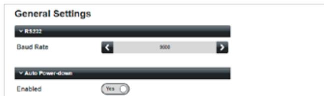
The default rate is 9600. Use the **Baud Rate** selector to set an alternative rate; the available options are 4800, 19200, 38400, 57600 and 115200.
