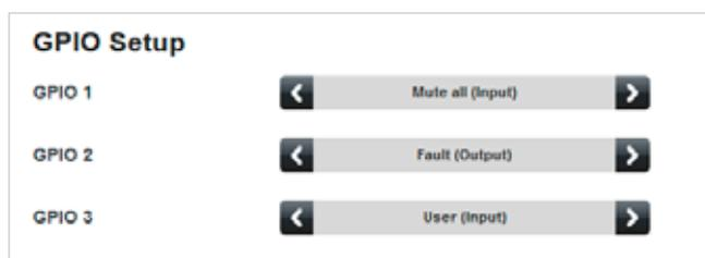
The port has three separate pins (GPIO 1, GPIO 2 and GPIO 3), each which may be configured in one of four ways – two input options and two output options. See "The GPIO Port" on page 48 for electrical and connection details of the GPIO port.
