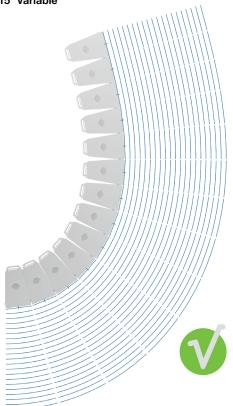
With the VC LINE, the vertical dispersion can be adjusted according to the splay angle between the individual elements, creating a seamless connection between the wavefronts of the elements. The result is a homogeneous wavefront and no comb filter effect.
