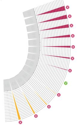
With conventional line arrays, the non-adjustable vertical dispersion leads to an overlap of the wavefront at all splay angles except the angle corresponding to the nominal vertical dispersion, in our example 10°. This leads to a phase shift within the wavefront, which in turn leads to the dreaded comb filter effect. If the splay angle exceeds the nominal angle (if the enclosure allows this), imperfections in the wavefront occur. This leads to dips in the frequency response.
